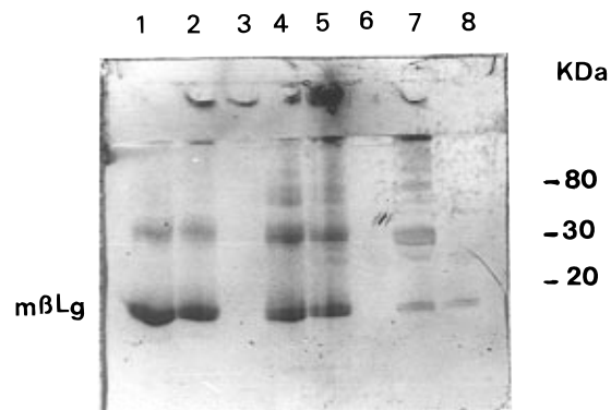
Figure 4. Immunoblot with antiserum against \beta -Lg of a SDS-PAGE plate under nonreducing conditions: lane 1, \beta -Lg; lane 2, a mixture of \kappa -casein and \beta -Lg; lane 3, \kappa -casein; lane 4, \beta -Lg pressurized at 400 MPa for 30 min; lane 5, a mixture of \kappa -casein and \beta -Lg pressurized at 400 MPa for 30 min; lane 6, \kappa -casein pressurized at 400 MPa for 30 min; lane 7, protein precipitated at pH 4.6 from milk pressurized at 400 MPa for 30 min; lane 8, protein precipitated at pH 4.6 from raw milk. m\beta -Lg = monomeric \beta -Lg.
